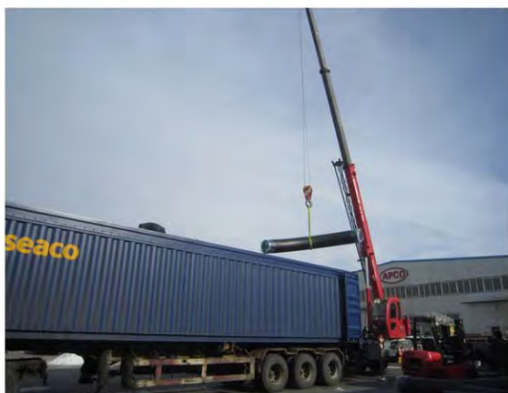
Hot Induction Bneds Being loaded
